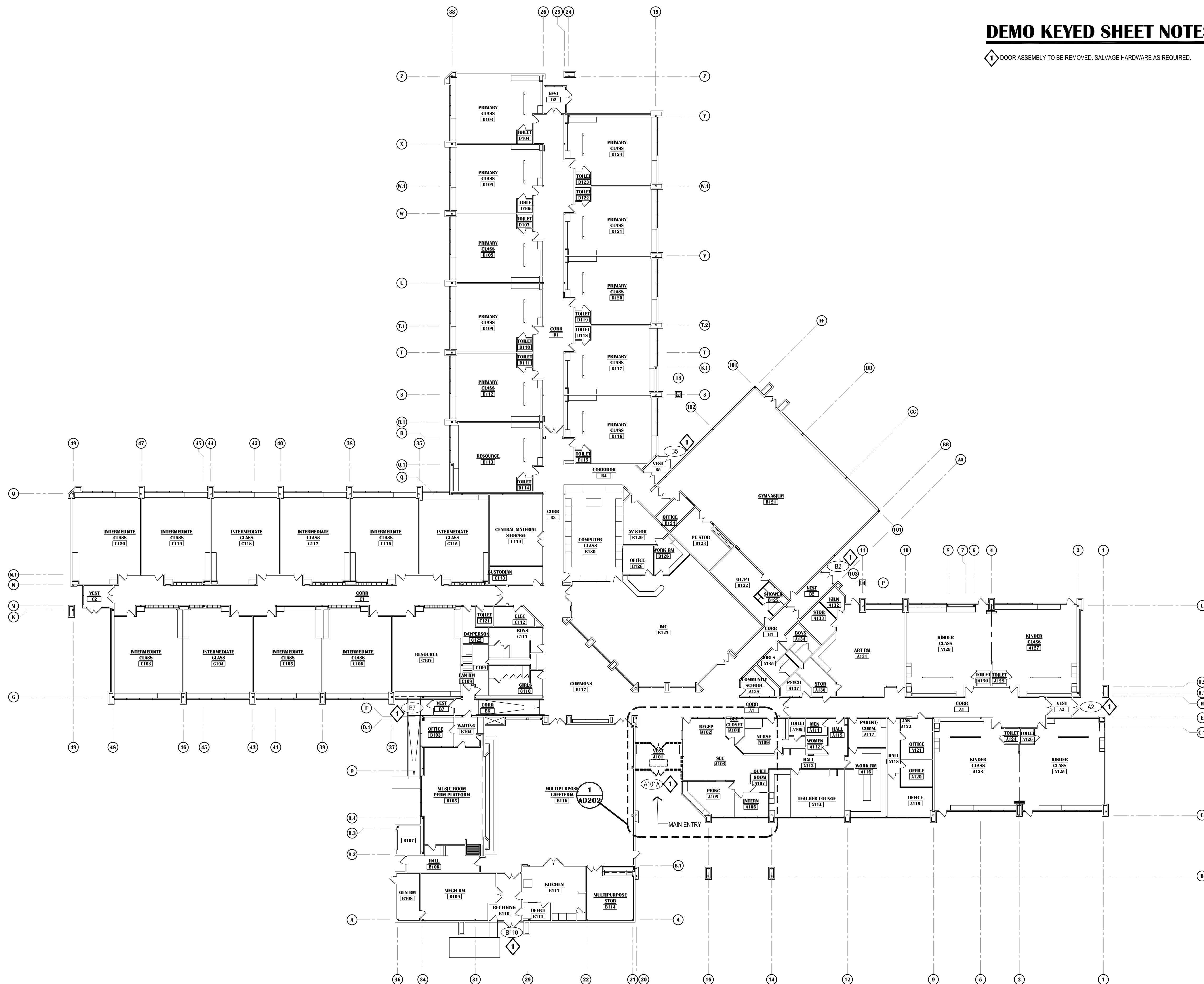
1 OVERALL FLOOR PLAN - DEMOLITION SCALE: 1"=20'
