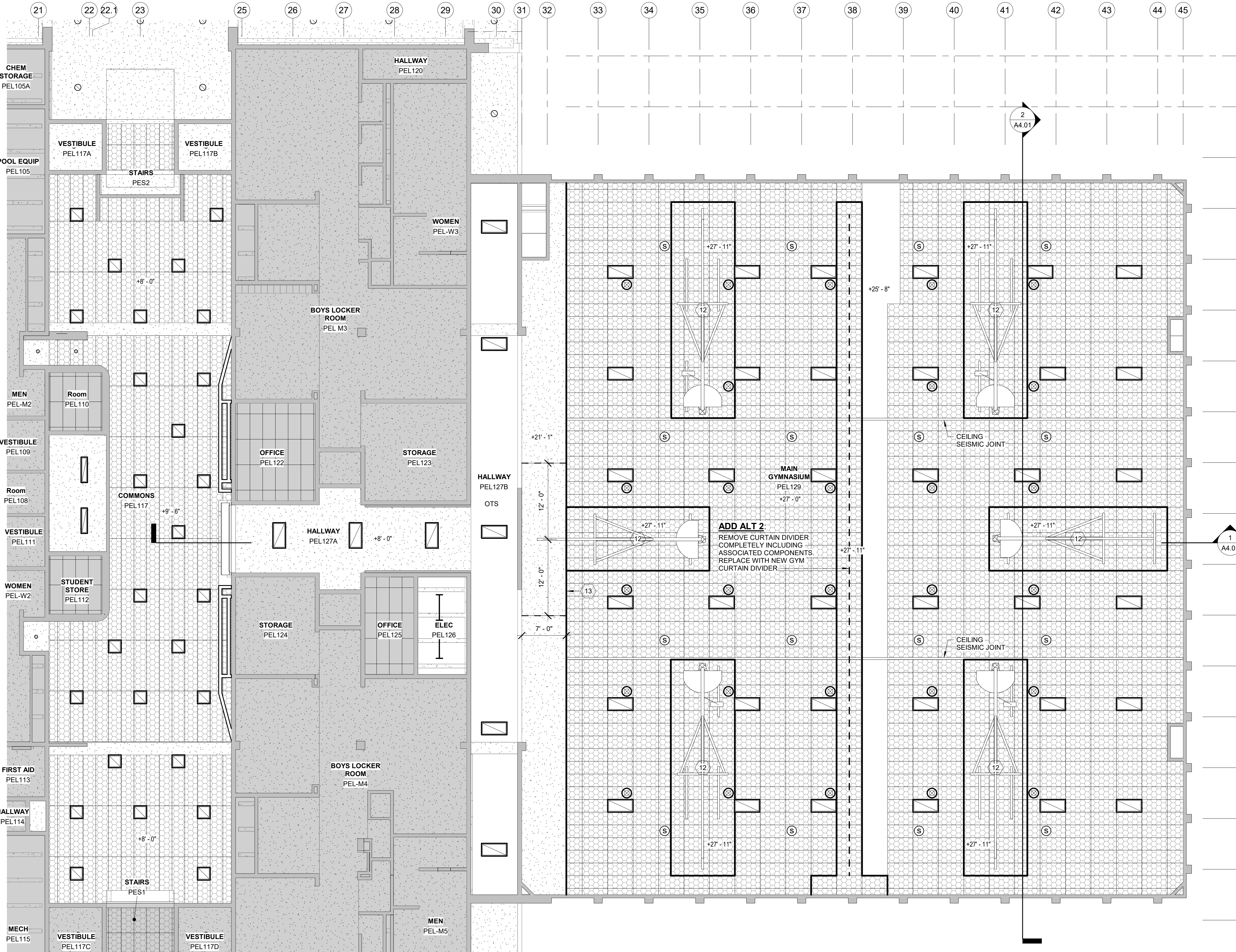
1 RCP - LEVEL 0 - GYM AND COMMONS A2.01 SCALE: 1/8" = 1'-0"
