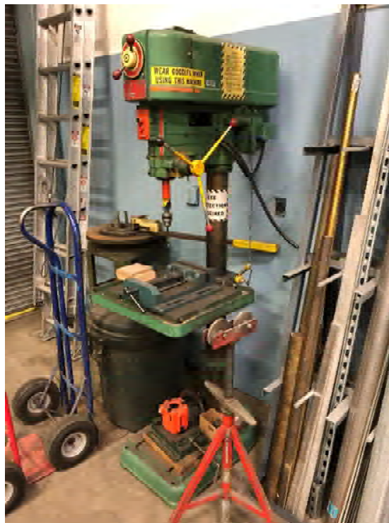
Welding Shop, Unrestrained Equipment Figure B- 94
