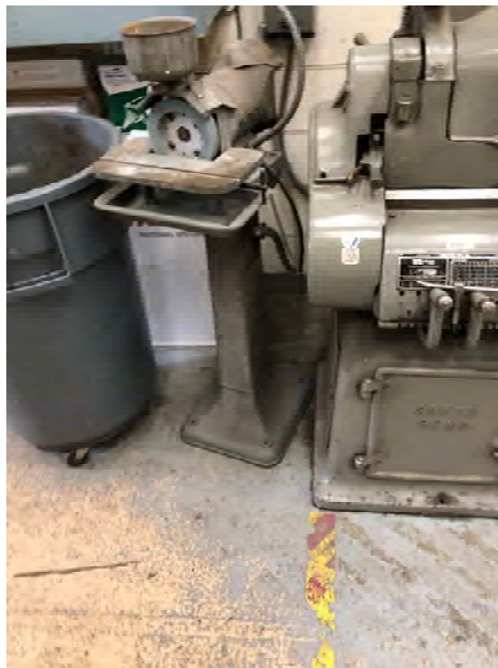
Welding Shop, Unrestrained Equipment Figure B- 92
