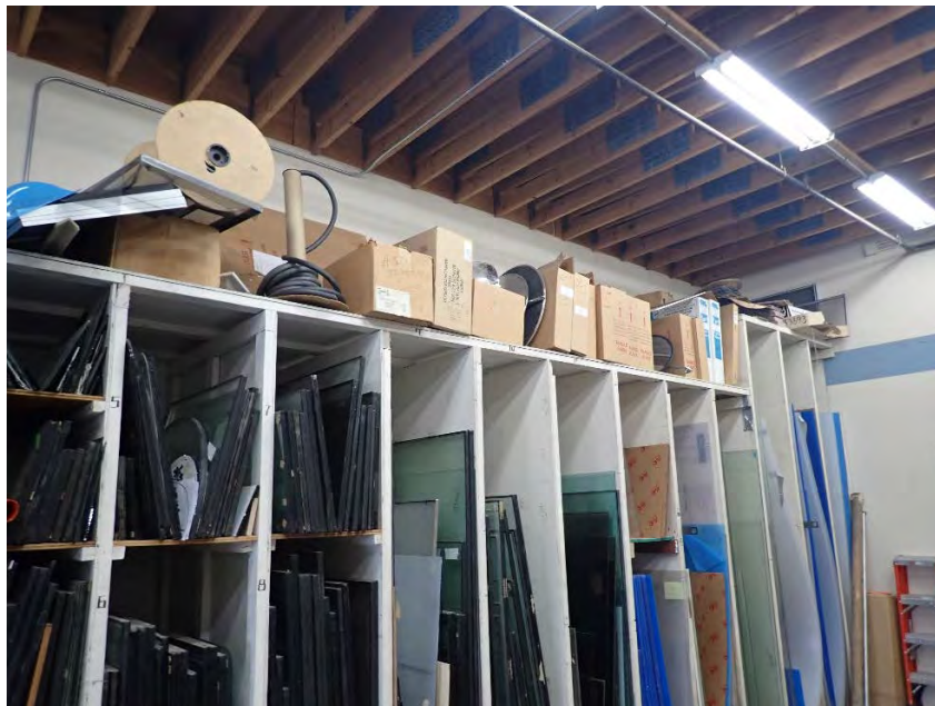
Glass Shop, Fall Prone Contents Figure B- 32
