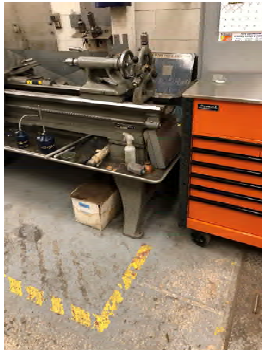
Welding Shop, Unrestrained Equipment Figure B- 91
