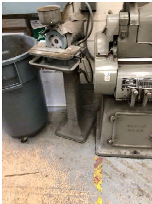
Welding Shop, Unrestrained Equipment Figure B- 92
