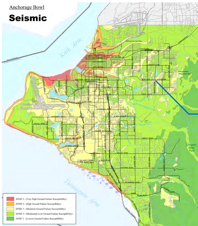
Figure 4 - Ground Failure Susceptibility Map, Municipality of Anchorage, 2006.
