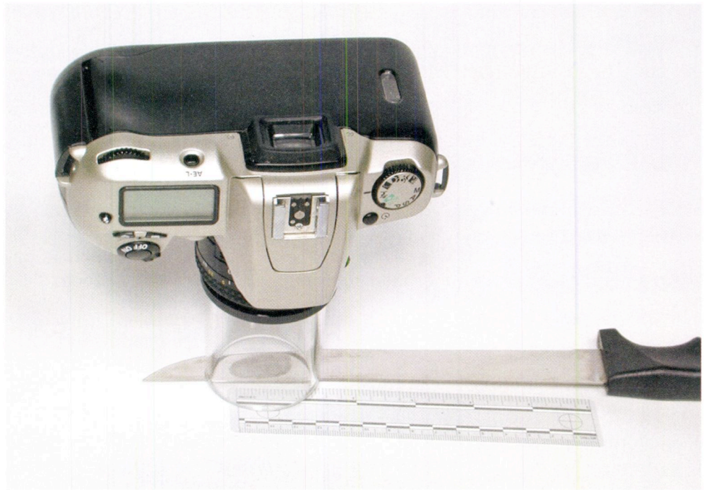
FIGURE 14-19 Camera fitted with an adapter designed to give an approximate 1:1 photograph of a fingerprint. Courtesy Sirchie Finger Print Laboratories, Inc., Youngsville, N.C., www.sirchie.com
