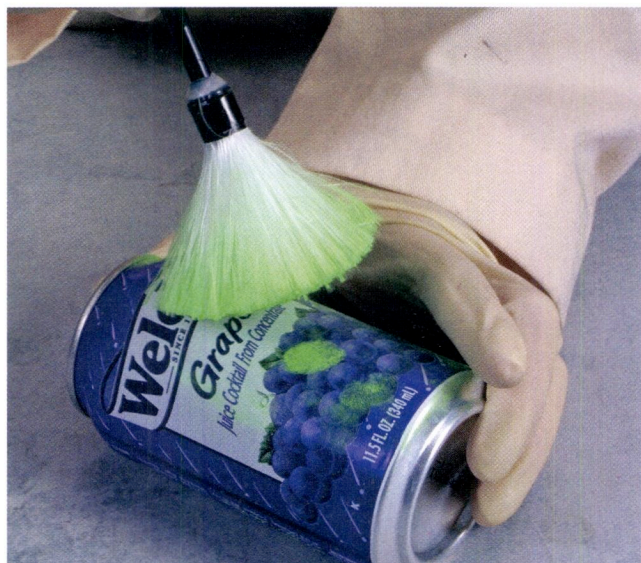
FIGURE 14-12 Developing a latent fingerprint on a surface by applying a fingerprint powder with a fiberglass brush. Courtesy Sirchie Finger Print Laboratories, Inc., Youngsville, N.C., www.sirchie.com
